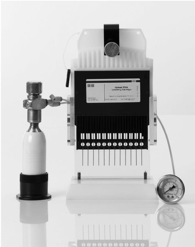
**D4. Slowly adjust the pressure to 60–65 psi, monitoring the pressure displayed in the pressure gauge.**
